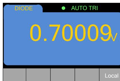
Figure 2.6.1 Diode measurement interface
