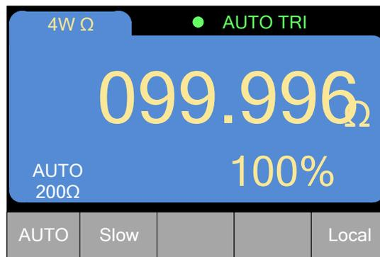
Figure 2.3.3 4-wire resistance measurement interface
